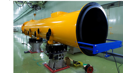
Figure 6 cross-section of STF Phase 1 cryomodule. Top-left is for TESLA-shape cavities, top-right is for LL-shape cavities. Middle is for two 5m cryostat connected. And down is the picture of cryostat.
