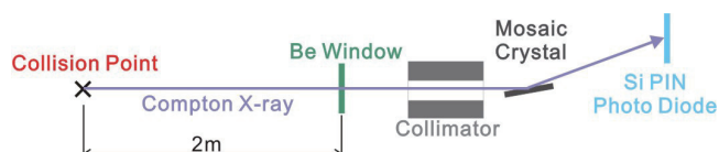
Fig.3.3 : Schematic of X-ray Detector at LUCX
