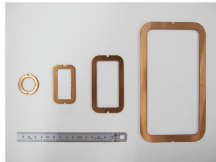
Figure 3: Gaskets, material: oxygen free copper, hardness: Hv 90, thickness: 2mm (Start from the Left: Hybrid Flange, C-band ADESY Flange, S-band ADESY Flange, L-band ADESY Flange)
