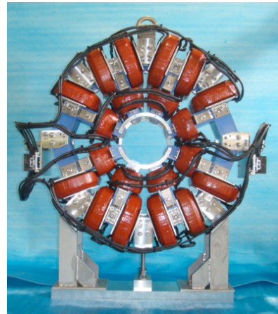
Fig. 5: Magnet assembly. The ring at the top will be replaced by an alignment base.
