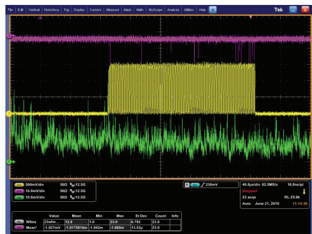
Figure 1: Signals from a plastic scintillation counter (magenta) and a Ar- CO_2 proportional counter (green) at SDTL13 section. The beam current signal with a current transformer is also shown (yellow).
