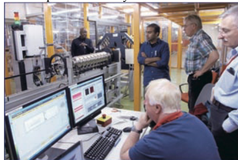
Figure 4: Installation team from FNAL has started up the cavity-tuning machine at STF.
