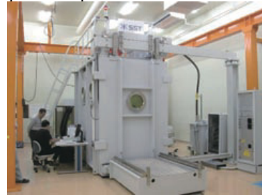
Figure 7: EBW machine commissioning at Cavity Fabrication Facility.
