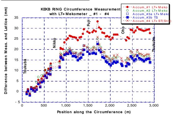
Figure 2: Accumulation of dL (difference between measurement and designed value)
