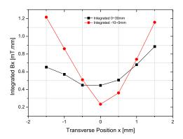
Figure 9: Integrated transverse magnetic field  $B_x$  along z for spiral slit FC.
