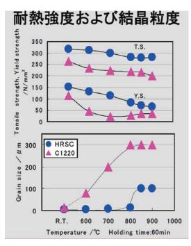
Figure 3: The comparison of the grain size, tensile strength and yield strength for HRSC and OFC at various temperature.
