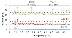
Figure 3: Frequency spectra for 0.21, 0.55, and 1.3 ps bunch lengths. Factors and offsets were adjusted for comparison. The theoretical frequencies for  $TM_{0n}$  modes (cross) according to Eq. (1) were shown.
