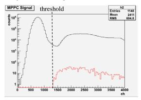
Figure 5: ADC Signal of MPPC during beam test
