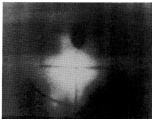
Fig. 2 A TV image of the beam on the screen with a hole at the center. There are vertical and horizontal reference lines at intervals of 5 mm on the screen. The beam was shifted from the center of the screen to avoid the hole.
