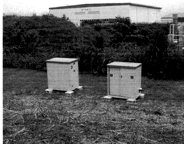
Fig. 1 The earth shields of the KEK 12-GeV PS. Neutron rem-counters are placed in the containers.
